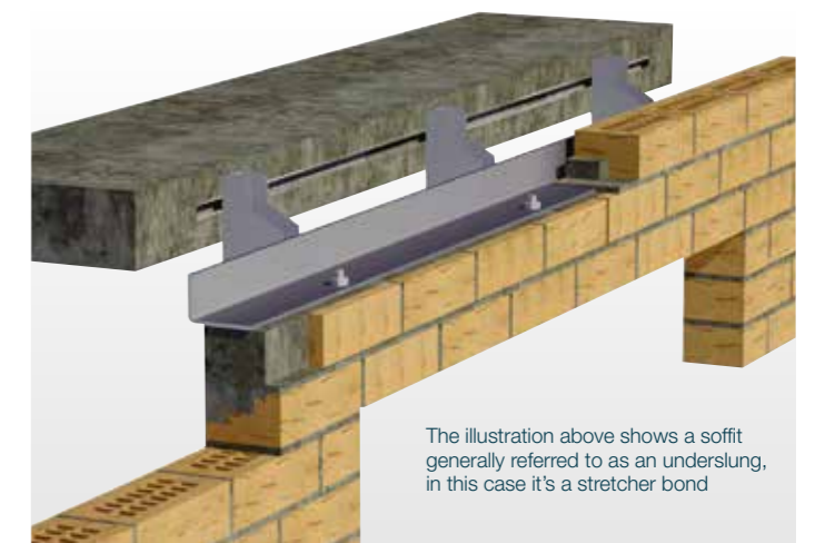
Underslung brick-faced soffits
