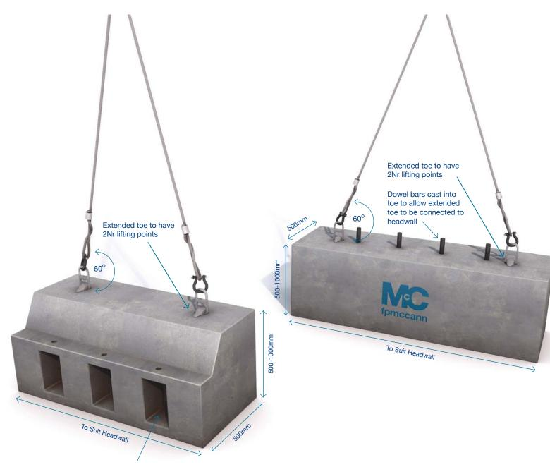
210x125mm holes to allow extended toe to be connected to headwall. Void filled on site by others
