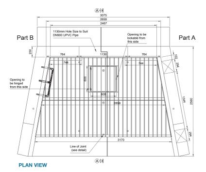
XXL T3 Headwall 1130mm hole to suit 900 pipe Special Grate with hinged access Ladders
