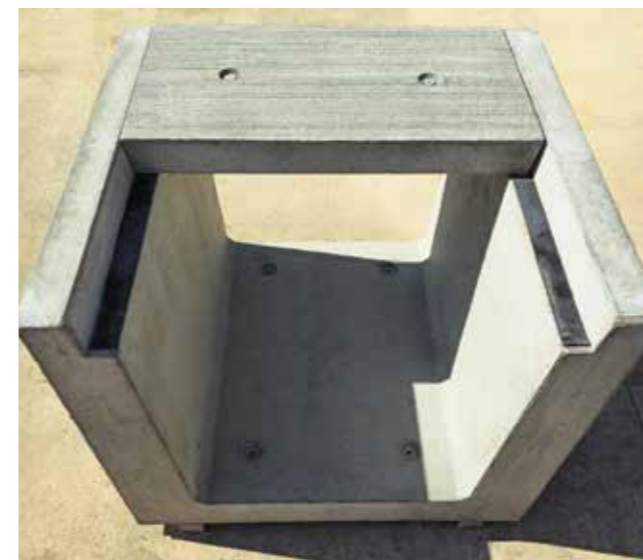
5. Rubber membrane is required underneath all concrete lids. Minimum thickness of 2mm to reduce noise and vibration effects.
