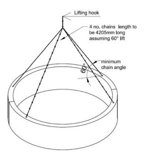
Unit weight and identification of lifting points will be marked on each casting for information.
