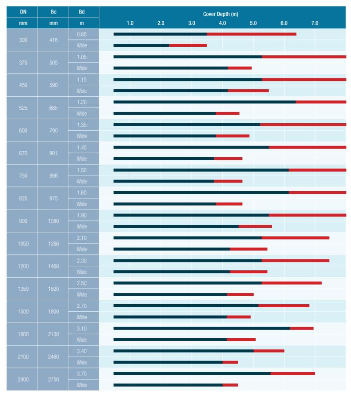
DN = Nominal diameter Bc = External diameter Bd = Trench width
