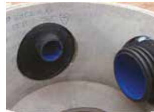
Once pipe is fitted to the connector, up to 45° of deflection is possible without breaking the seal.
