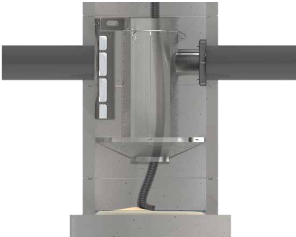
Figure 6 - Vacuum Truck hose in the settled sediment sump region (Internal Assembly rendered transparent for visualization)
