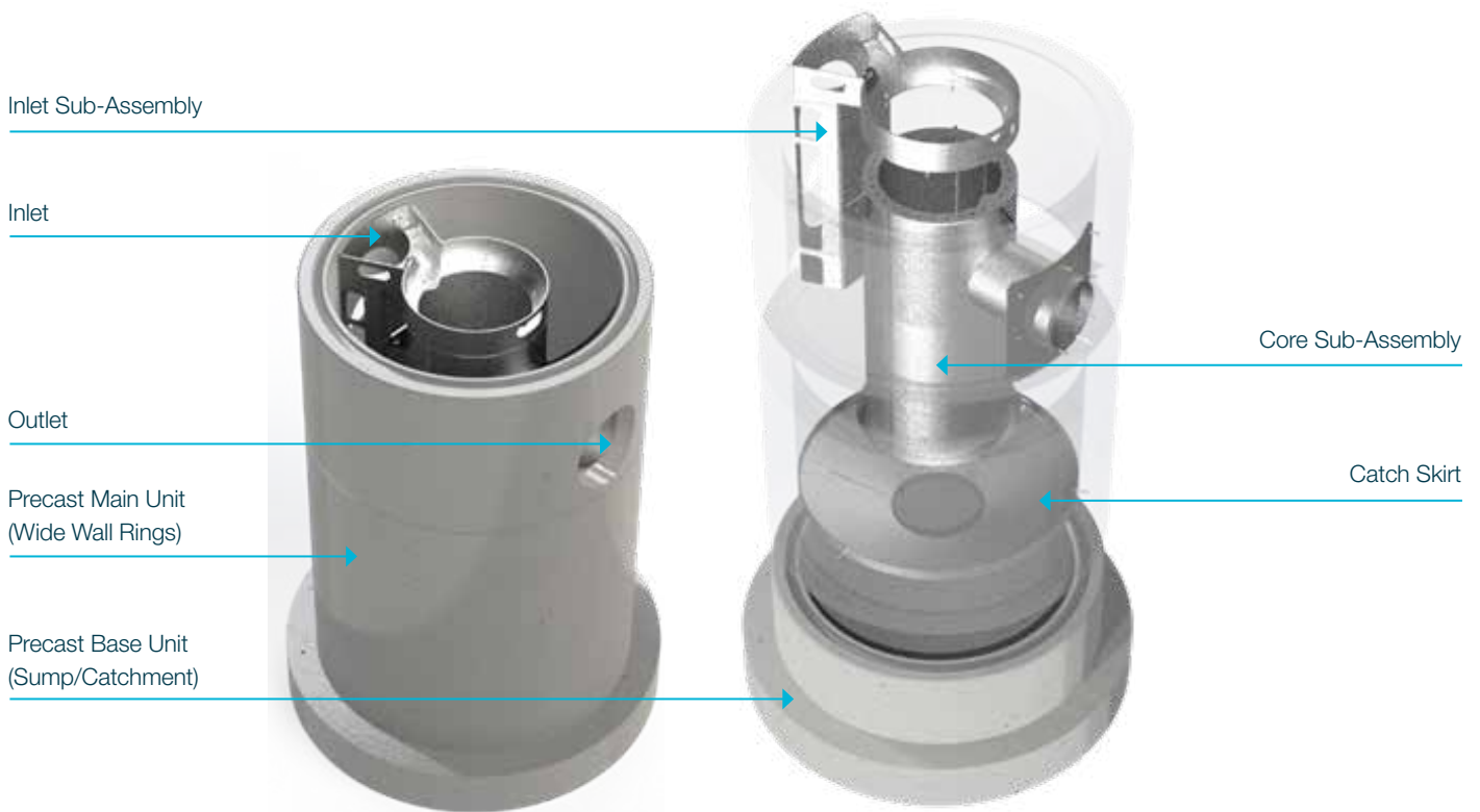
Figure 1 - StormCleanser™ Assembly and Exploded View
