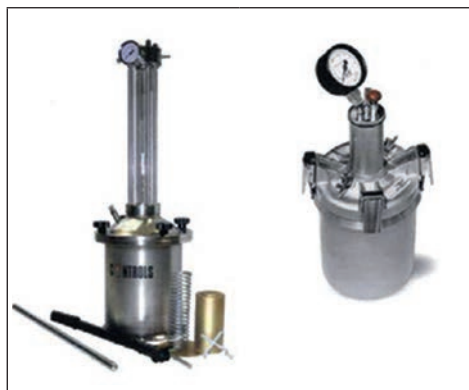
Fig C.1 Water column test apparatus
