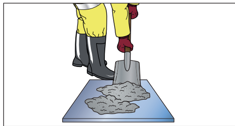
Figure B.1 Remixing sample on tray
