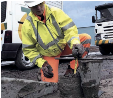
Figure A.1 Sampling from concrete stream
