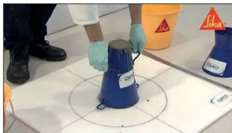
Figure B.11 Slump-flow cone ready for lifting
