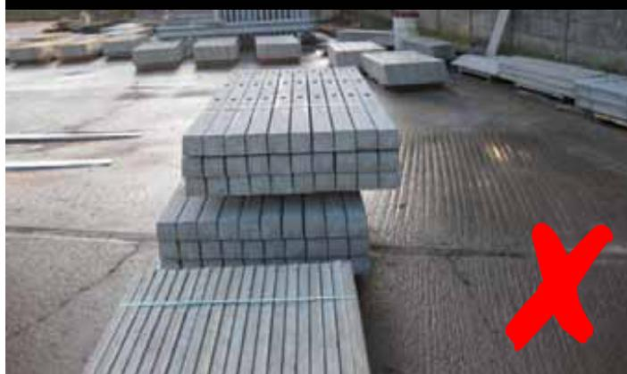
**Products must not be stacked on top of each other like this as the load bearers are not in line**
